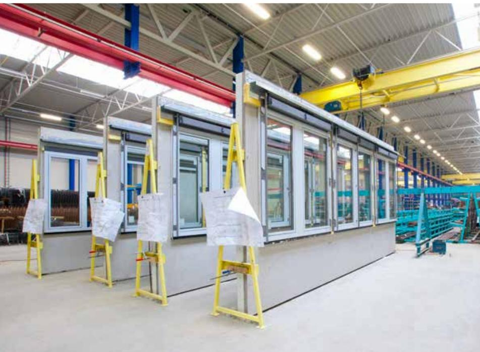
Hybrid constructions, such as our external wall elements, enable fast construction times and high quality.
